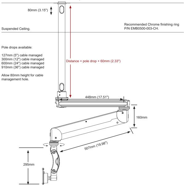
The specifying guide above is designed to assist in determining the most appropriate length of pole drop. The EMT2EQ LCD ceiling mount is suitable for use within many medical based environments including OR theatres, EPRS, and ward based patient use and therefore it's not possible to provide a single recommended height due to the varying nature of each application.
